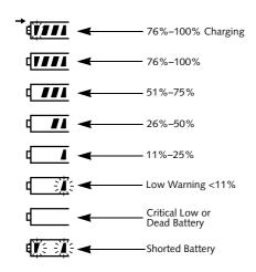
Figure 2-12 Battery Level Indicator
